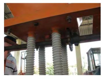
A view from the underside showing the drive mechanism for the horizontal plate. Apparently each plate meters seed to four outlets. Patrice Autfray (who is a member of the CIRAD team in Laos) has sent me some pictures of the ARC Gongli 2WT seed drill being tried out in Laos. I recently sent a pair of staggered double disc openers to Patrice to test in very heavy mulch (SCV) systems there. He reports:
