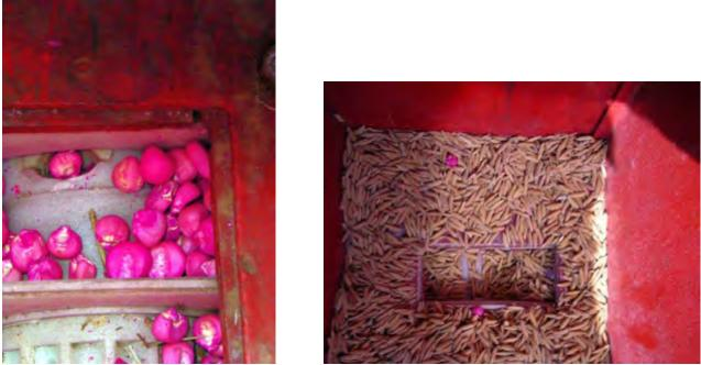
Metering maize though the large flute option and rice through the small grain option.
