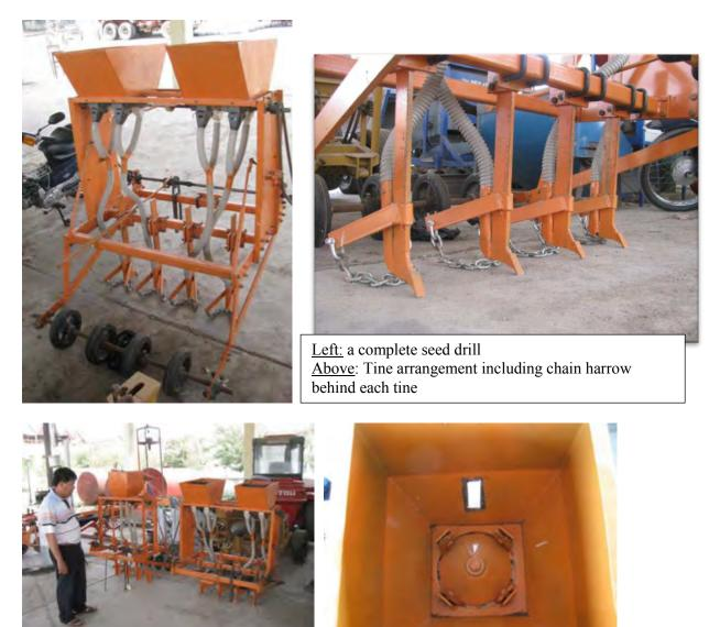
Left: Two seed drills, the one on the right with traditional seed boxes and the one on the left with a locally made horizontal plate metering system.
