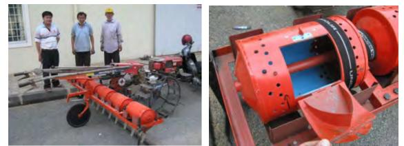
Left: Messrs Chea Sovandina, Prum Cham Roeun and Chuon Sarom of GDA DAEng who developed the 2WT powered drum seeder prototype. <u>Right:</u> Close view of the drum with inner agitator
