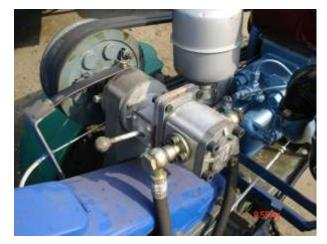
This PTO is coupled to a hydraulic pump. The hydraulic unit is used to power a power operated tilt hydraulic ram, when a tilt trailer is operated with a 2WT.
