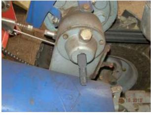
I have suggested to Mr. Sun that a PTO similar to that shown on the left may be an alternative. I have photo shopped a PTO shaft to the clutch section of a Dong Feng 2WT.
