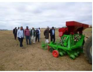
Angled single disc as fitted to seed drill on 4WT Note how the disc units are 'pushed'
