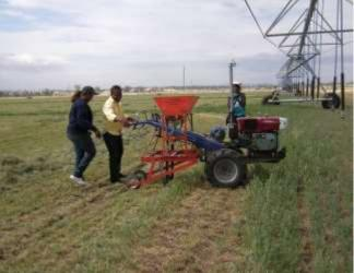
The unit was set up in a two row configuration, for row crop planting, although it is capable of planting up to four rows of close drilled crops. It had no difficulty planting into the light residue conditions with cut lucerne plants
